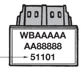
If this is no longer possible, the coding plug must be removed in order to read the code on the label of the coding plug.
